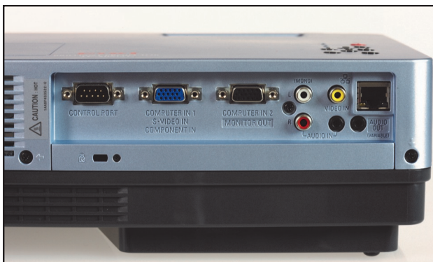
An example of the various connection types found on a projector
