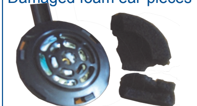
Damaged foam ear-pieces
