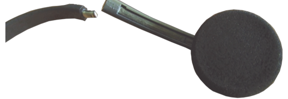
Snapped, thin head frames
