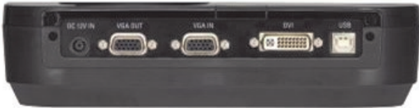
An example of the various connection types found on a mid-range visualiser
